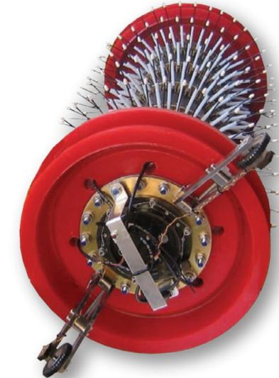
Unique concepts behind tool design, analysis and data management software allow the Porcupine as a "stand alone" tool or combined with MFL modules in a single ILI tool, able to do internal and external inspection in a single passage.
